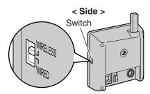
When you switch from WIRED to WIRELESS or vice versa, restart the camera. Some routers may also need to be restarted after switching.
